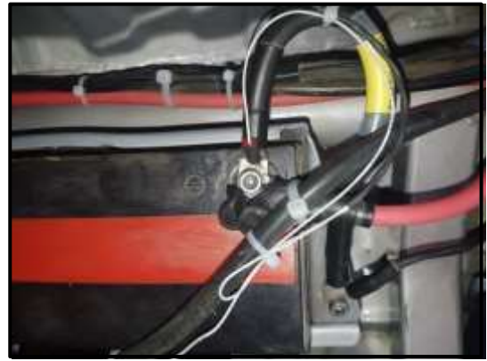
Permanent Power & Earth Connections
