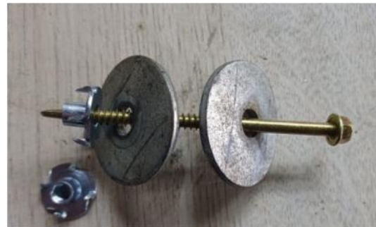
Tek Screw that may be used for tyre walls. Nut in right side photo from Gelmar
