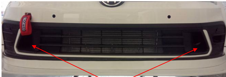
Brake Duct inlets
