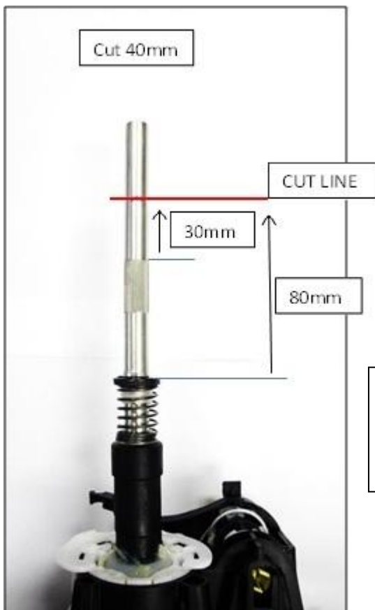
Gearshift may be cut 40mm or the gear knob inside may be drilled to lower the knob position for driver comfort.
