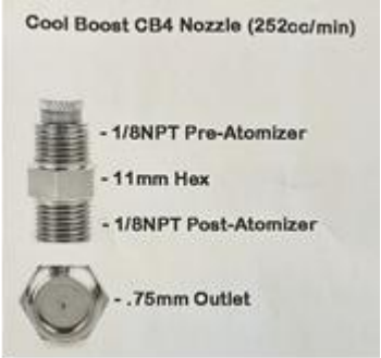
Number of spray nozzles: 8 Spray nozzle hole size: Diameter 0.75 mm is the biggest size allowed.
