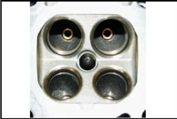
C8-7) Combustion chamber
