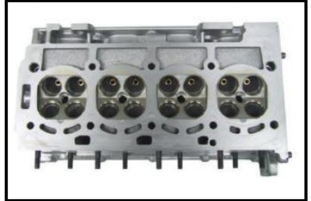
C8-2) Bare cylinderhead seen from underneath (chamber side)
