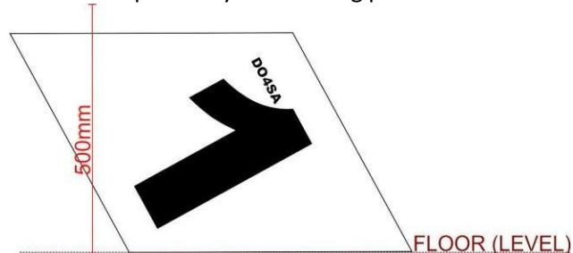
D. Attempting to measure it any other way will result in measurements of e.g. 540mm. Always remember to measure as if the bottom of your measurement is lying on the floor on you are measuring from the floor upwards.
