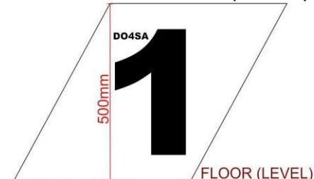
C. Now you can turn the wing onto its other side (or simply use your level on the other side if the wing is fitted to the car). GUIDE: ALWAYS USE THE FLOOR (OR LEVEL) along the bottom of the endplate as your starting point from which to measure.
