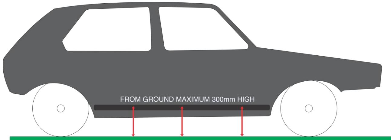
27.2 The wheel and body protector must be straight and only curve inwards at each end once mounted;
