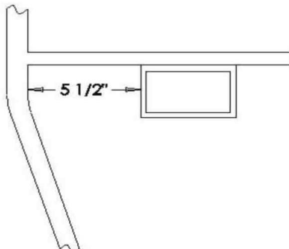
**Note:** The measurement for the battery box offset will be taken at the point closest to the crossmember, from the inside of the framerail to the outside of the battery box.
