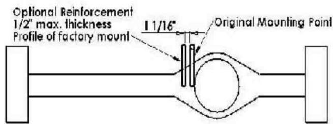
(This reinforcement will secure the opposite side of the rod end of the upper link)
