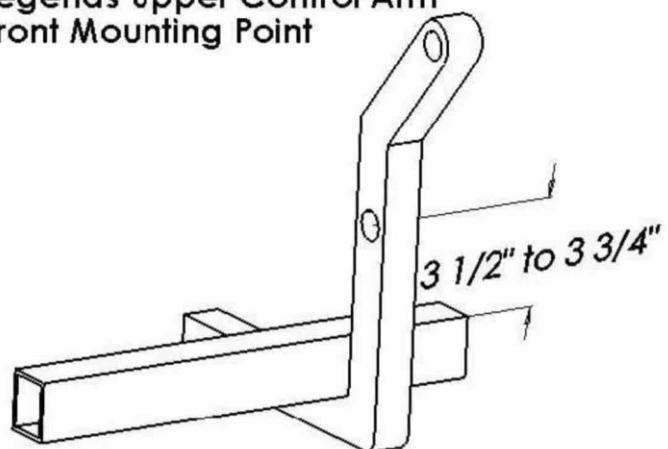
$3 \frac{1}{2}$ " to  $3 \frac{3}{4}$ " (from the top of the frame to the center of the pick-up point holes)
