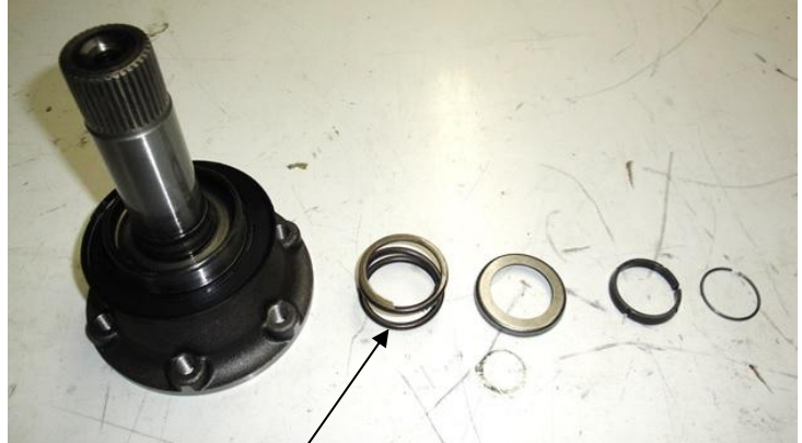
Spring L = 20.5 mm \pm 0.2 Wire Dia = 3.8 mm
