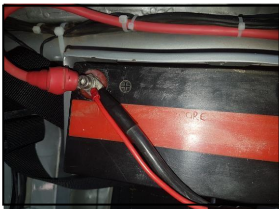
Permanent Power & Earth Connections
