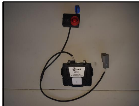
Panic Button Assembly & Ctrack Unit
