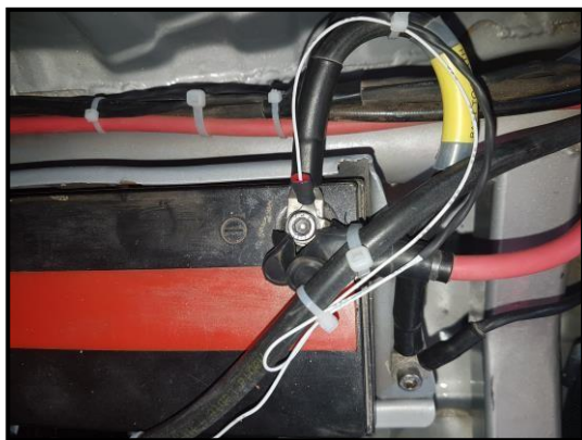
Permanent Power & Earth Connections
