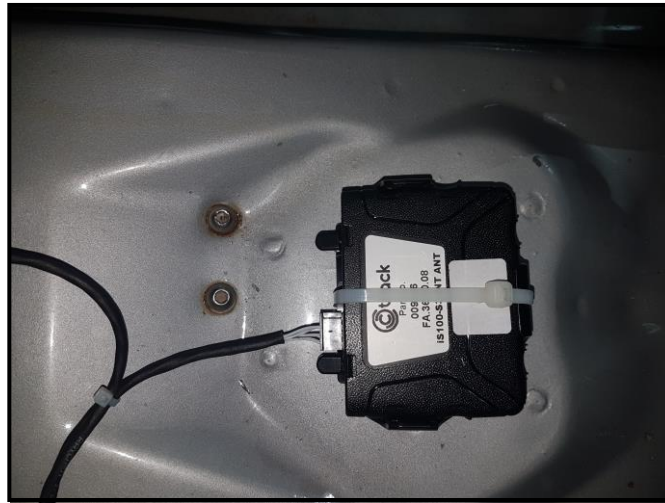
Securing the Ctrack Unit
