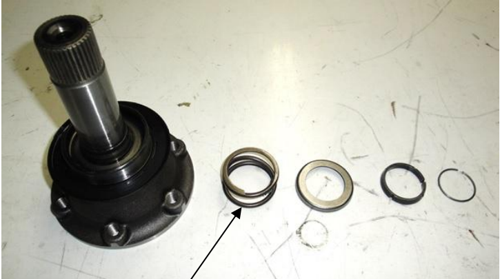
Spring L = 20.5 mm \pm 0.2 Wire Dia = 3.8 mm
