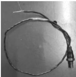
Temperature sensor NTC1- M8-S-10K-050-193 or TS-NTC3K-M8-14
