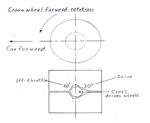
The limited slip differential must be run to the following specifications:
