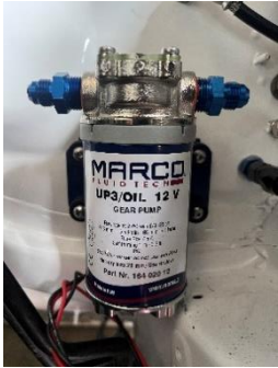
Gearbox Pump. Marco UP3/ Oil 12V
