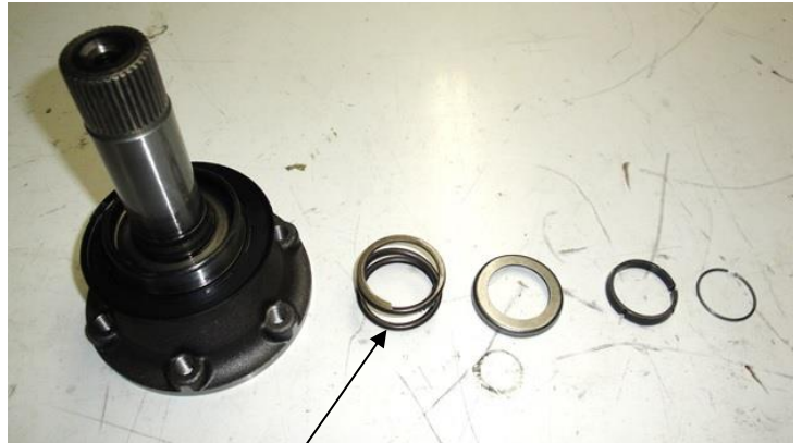
Spring L = 20.5 mm \pm 0.2 Wire Dia = 3.8 mm
