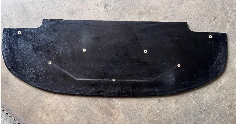
30.5. Front splitter board.
