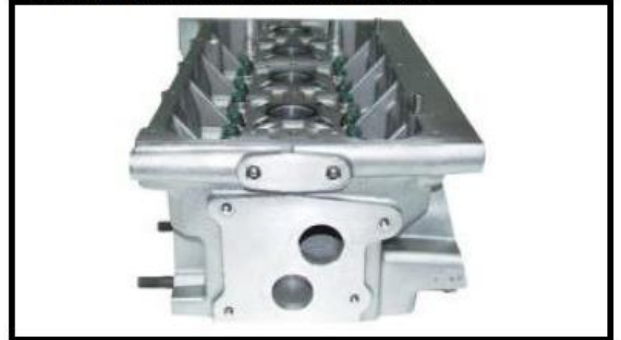
C8-6) Bare cylinderhead seen from flywheel side
