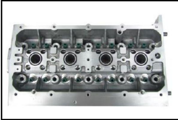
C8-1) Bare cylinderhead seen from top (camshaft side)
