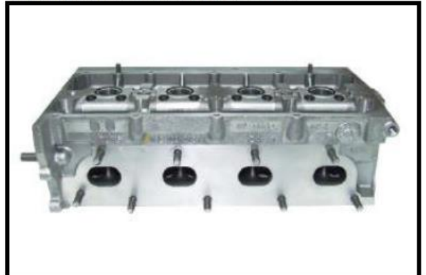
C8-4) Bare cylinderhead seen from exhaust side
