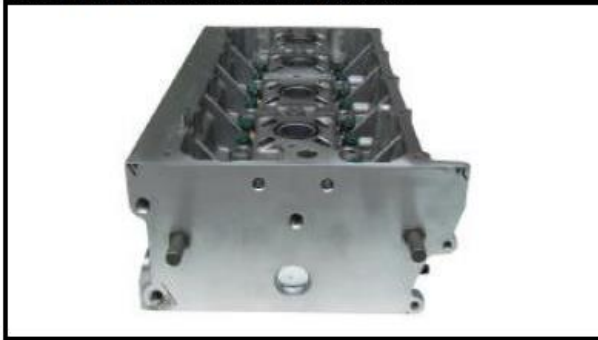
C8-5) Bare cylinderhead seen from timing side
