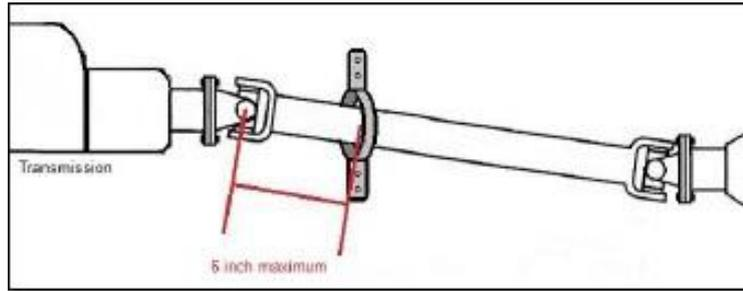
The driveshaft loop may be made of minimum 6.35mm steel x 50mm wide strap or 23mm x 1.65mm steel tubing and be securely mounted in case of universal joint failure.
