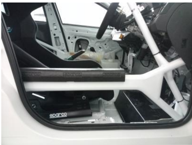
Door cross – Design 2 as per FIA Homologation Regulations – Safety Cages. Drawing SC-11b
