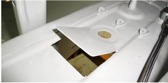
Cut-out made in tunnel for gearshift cables to pass through.
