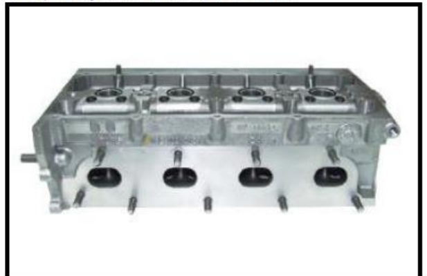
C8-4) Bare cylinderhead seen from exhaust side
