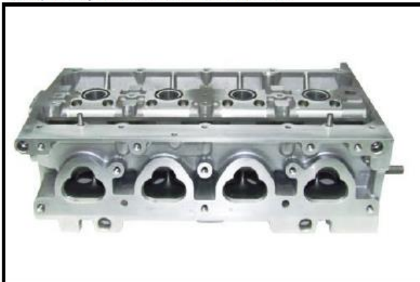
C8-3) Bare cylinderhead seen from intake side
