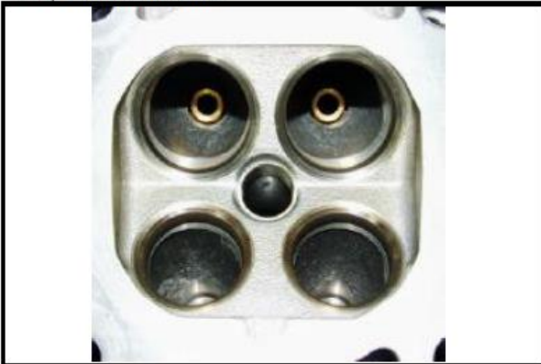
C8-7) Combustion chamber
