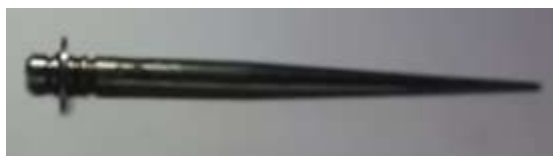
Needle clip position <2= for Kid Rok
