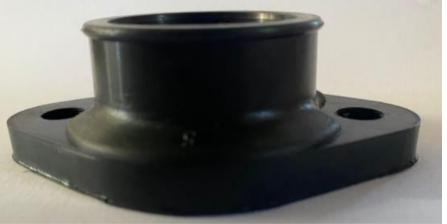
**i.** Exhaust Manifold: The only exhaust manifold permitted is as per photos and dimensions below. No material may be added or removed. The Exhaust Manifold gasket as supplied must be fitted at all times.
