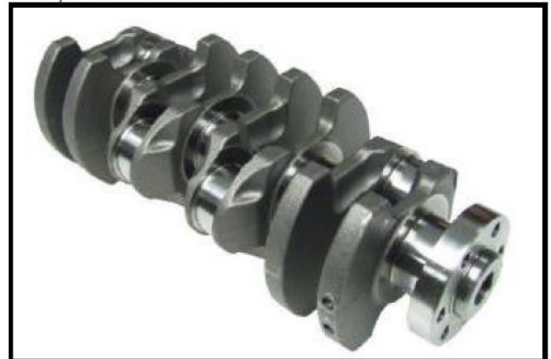
C6-2) Crankshaft from ¾ rear
