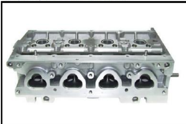
C8-3) Bare cylinderhead seen from intake side
