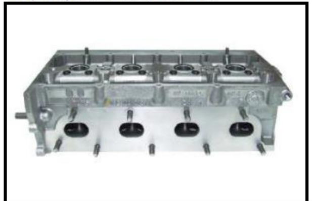
C8-4) Bare cylinderhead seen from exhaust side
