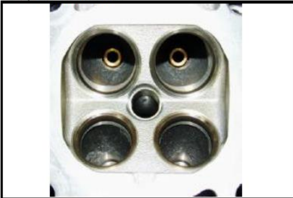
C8-7) Combustion chamber
