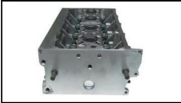
C8-5) Bare cylinderhead seen from timing side
