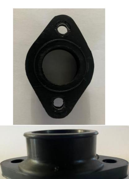
i. Exhaust Manifold: The only exhaust manifold permitted is as per photos and dimensions below. No material may be added or removed. The Exhaust Manifold gasket as supplied must be fitted at all times.
