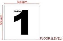
B. How do you take this measurement when the plate is not square? The same plate above has been skewed in the picture below. GUIDE: ALWAYS USE THE FLOOR (OR LEVEL) along the bottom of the endplate as your starting point from which to measure.
