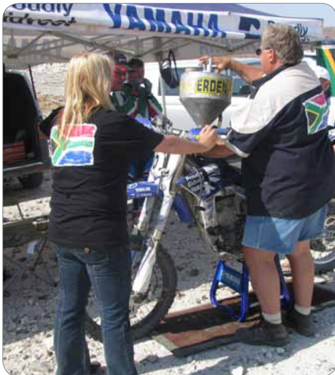
Above: The correct use of environmental mats at refueling points ensure that there is no pollution of water sources and soil.
