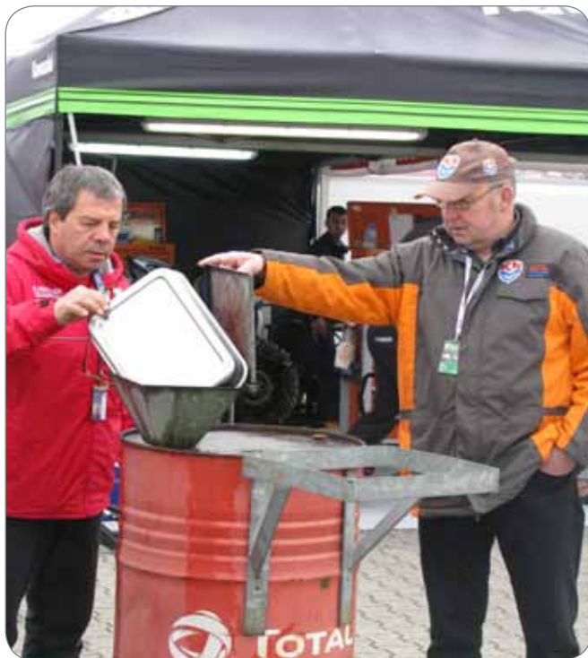
Above: Proper disposal in a waste fluid container with drip tray.
