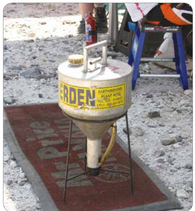
Above: The correct use of environmental mats at refueling points ensure that there is no pollution of water sources and soil.
