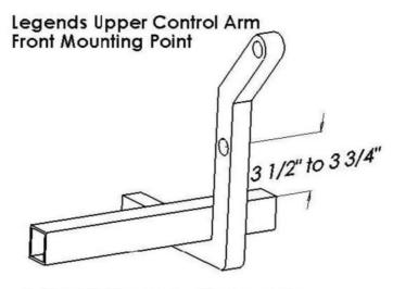
3 1/2" to 3 3/4" (from the top of the frame to the center of the pick-up point holes)
