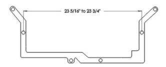
Legends Left Side Motor Mount Pickup Points & Front Clip Measurements
