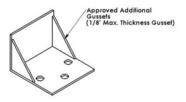
Upper Link Double Shear Mount (Chassis Side)
