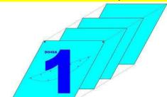
F. The inner plates should be contained within the confines of the endplates (as indicated by the dotted-line in diagram).
