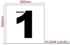
B. How do you take this measurement when the plate is not square? The same plate above has been skewed in the picture below. GUIDE: ALWAYS USE THE FLOOR (OR LEVEL) along the bottom of the endplate as your starting point from which to measure.
